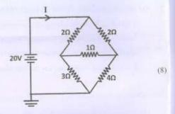
(b) Find out source current  $I_i$  and current through the resistance  $2\Omega$   $(I_{2\Omega})$  in the circuit given below.
