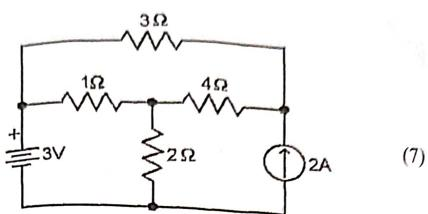
(b) Obtain Norton equivalent circuit for the network external to the  $3\Omega$  resistance for the given network. Further determine the current through  $3\Omega$  resistor.
