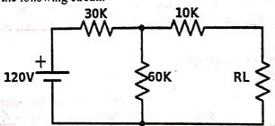
What is the power dissipated in  $R_L$  when matched?
