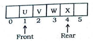
This Queue is implemented as a circular array. Show the contents of the Queue with the positions of Front and Rear after each of the following operations:
