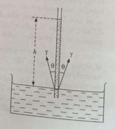
Fig. 2.4.4 Rise of a liquid in a capillary tube
