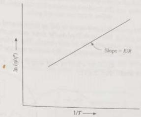
Fig. 2.3.4 Plot of  $\ln (\eta/\eta^{\circ})$ versus 1/T
