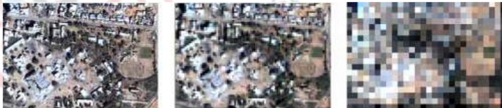
Fig. 10 Spatial resolution of an image: (Left) nominal 1m spatial resolution (middle) 5m spatial resolution (right) 30m spatial resolution.
