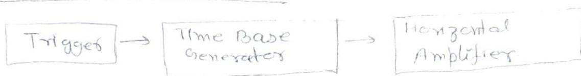
(a) Trigger circuit:- This circuit ensures that generation of the horizontal time-base (sweep) starts at the same point of the vertical input signal.
