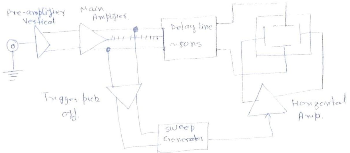
The horizontal signal (X-plate), (time base sweep voltage) is initiated or triggered by a portion of the input applied to the vertical CRT plates. Signal processing in the horizontal channel consists of generating and shaping a trigger pulse, that starts the sweep generator, whose output is fed to the horizontal amplifier and then to horizontal deflecting plates.
