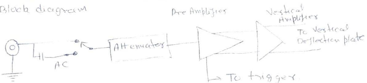
The main function of this system is to suitably amplify the input signal such that its basic characteristics do not undergo any change or modification. This has a switchable input coupling capacitor which helps to view the ac signal even within high voltage dc.
