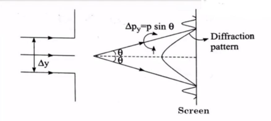
From the theory of diffraction for first order (n = 1) we have  $d \sin \theta = n\lambda$ Here in this case  $d = \Delta y$  and n = 1 so that,  $\Delta y . \sin \theta = \lambda$
