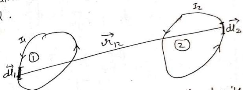
Consider two coils 1 & 2 and let a current  $I_1$  is pass through coil 1. Let  $\vec{B}_1$  denotes the mag. field due to this current in coil 1. Due to current  $I_1$ , a mag. flux  $\phi_{21}$  is associated with coil 2. ie
