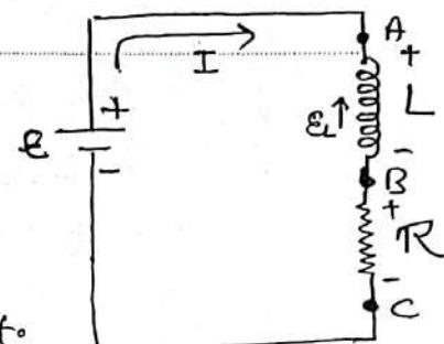
thus  $W = \frac{1}{2} L I^2$  is the energy required from an external source to overcome the emf in the inductance when the current rises to its steady value.
