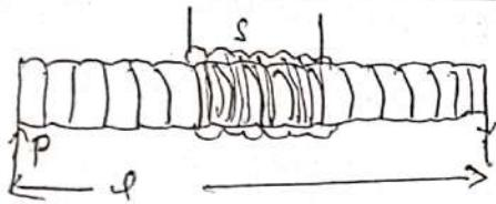
consider the secondary coils wound on the central part of primary coil P having an air core.
