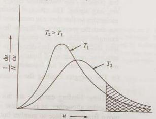
Fig. 2.2.2 Distribution of speeds of molecules
