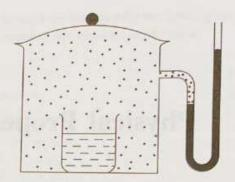
Fig. 2.2.1 Vapour pressure of a liquid
