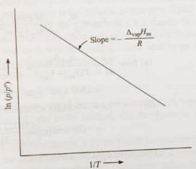
Fig. 2.2.5 Plot of  $\ln (p/p^{\circ})$  versus 1/T
