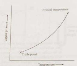
Fig. 2.2.4 Variation of vapour pressure with temperature
