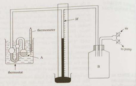
Fig. 2.2.6 The isoteniscope method for the measurement of vapour pressure
