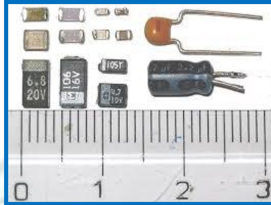
Figure 4: Comparison of discrete and SMD component sizes
