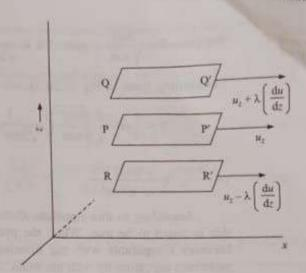
Fig. 1.20.1 Display of velocity gradient with the height of layer
