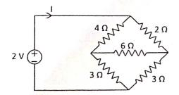
4. Using mesh analysis, determine the currents of the network in Fig.
