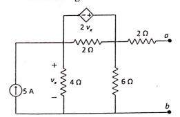
Find the Norton equivalent circuit for the portion of the network to the left of a-b in Fig.
