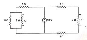
2. Write the mesh equations for the network in the Fig
