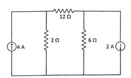
**6.** Find the Thevenin equivalent of the circuit in Fig. at terminals *a-h*.
