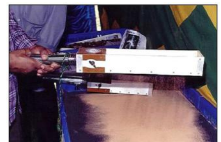
Battery Operated Duster for dusting disinfectants on rearing beds
