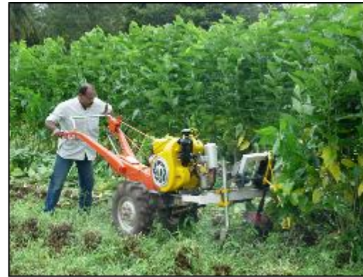
Power tiller operated mulberry shoot harvester (harvests 1000-1200 kg shoots per hour)
