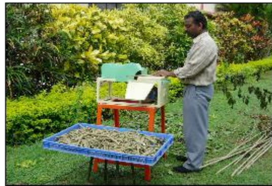
With help of mulberry cutting preparation machine developed by CSRTI, Mysore 1,400 to 1,500 cuttings can be prepared in one hour.
